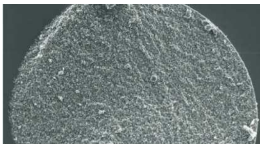
FE-SEM picture of a cut through a Kromasil 300 Å particle at 5 000 x magnification.
